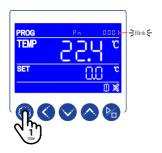
• Press the SETTING key 1 time to scroll through parameters until the parameter Cy appears.
