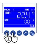
Press the SETTING and SHIFT keys for 3 seconds to enter the controller's internal parameter settings. The Time area will change and first digit will blink.
