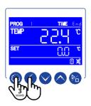
• Press the SETTING and SHIFT keys for 3 seconds to enter the controller's internal parameter settings. Time area will change and **fi**rst digit will blink.
