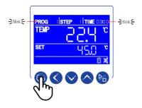
• Press the SETTING key to accept temperature setpoint. The **fi**rst TIME digit will blink.
