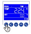
• Press the SETTING key for 3 seconds. "PROG 1" will initially blink. Then the number will blink.
