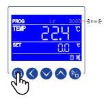
• Press the SETTING key to enter Level 1 parameters.
