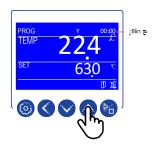
• Press the INCREASE key to enter the **fi**rst time value. Press the SHIFT key to move to the second cycle digit. Digit will blink. Press the INCREASE key to enter the second time value.
