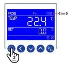
• Press the SETTING key 2 times to scroll through parameters until the parameter dy appears.
