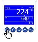
• Press the SETTING key 1 time to set parameter dy and return to the multi-step program standard state.
