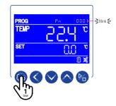
• Press the SETTING key 1 time to scroll through parameters until the parameter Cy appears.
