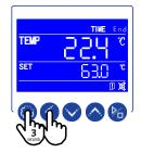
• Press and hold the SETTING and shift keys for 3 seconds to view the controller's internal parameters.
