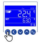
• Press the SETTING key 1 time to set parameter Mo and return to standard state.
