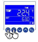
• Press the SETTING and SHIFT keys for 3 seconds to enter the controller's internal parameter settings. The time area will change and **fi**rst digit will blink.
