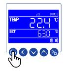
• Press the SETTING key 1 time to set parameter dy and return to **fi**xed value program standard state.
