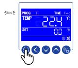
• Press the SETTING key to confirm the program to run.
