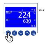
• The tM parameter will appear. Press the SETTING key 1 time to scroll through parameters until the parameter Po appears.
