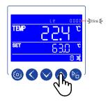
• Press the SETTING key to enter Level 1 parameters.
